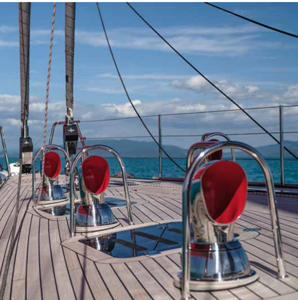
With the owner's emphasis on self-reliance, all-weather performance and minimal engine and generator hours, the standard flush decks feature full dorade ventilation and traveller in place of a single-point main for optimised sail trim. The skipper's simple seating swings up to stow away on the fixed bimini legs
