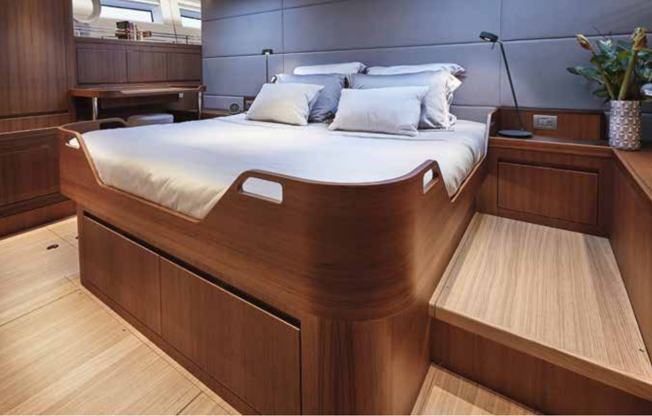
The single-section surround to the aft master suite bed (left) illustrates the technically complex joinery work. Safety features include life jacket lockers by all cabin exits, a snug galley with centreline refrigeration, high-sided beds with handholds and canting bases, practical sliding doors for corridor cupboards and saloon nav-comm station, which is duplicated in the crew quarters
