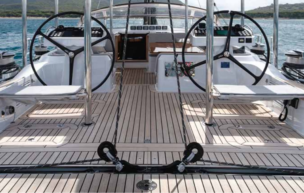
With the owner's emphasis on self-reliance, all-weather performance and minimal engine and generator hours, the standard flush decks feature full dorade ventilation and traveller in place of a single-point main for optimised sail trim. The skipper's simple seating swings up to stow away on the fixed bimini legs
