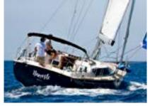
MAIN DIMENSIONS 42CS Length overall 12.85 m Length waterline Maximum beam Displacement 11.76 m 4.15 m 11,000 kg
